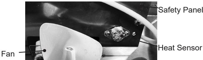
6. Reach around the safety panel and press the reset button (see photo to the right).
